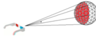
(b) For each viewpoint taken by the participant, we increment a value associated to each visible triangle by the duration spent on this viewpoint.
