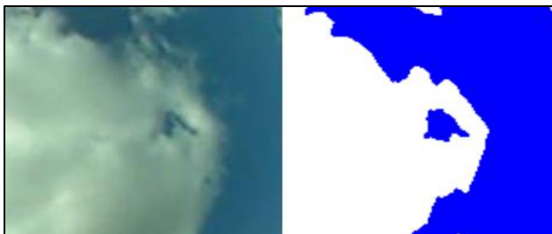
Figure 4: A portion of a Total Sky Imager (TSI) image and segmentation into cloud and non-cloud pixels.
